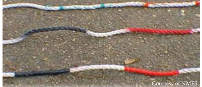
Shown are three simple methods to create 12" red marks. Top: colored twine is seized around the line and woven between the strands. Center: dry line is spray-painted. Bottom: colored electrical tape wrapped in one direction and then back over itself to form two layers. Not shown: wire tie or twine woven between rope strands, dyed rope, plastic or heat shrink tubing or other methods approved by NMFS.
